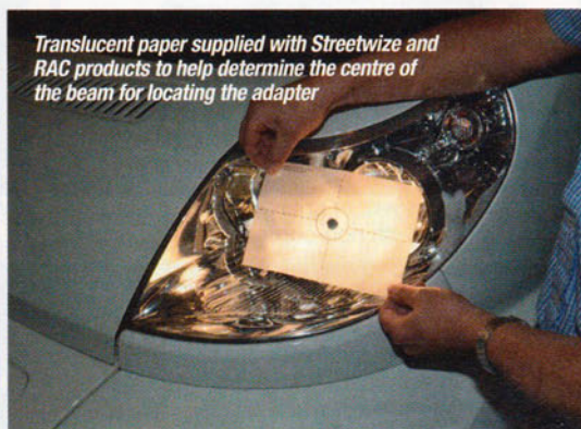
Adaptor with clear tape used to position adaptor for optimum performance for test purposes
