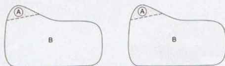
Headlamp beam pattern showing "kick-up" area A which needs to be masked to eliminate glare to oncoming drivers on the Continent
