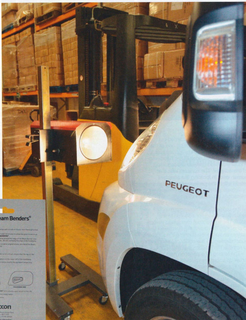
Using a borrowed headlamp alignment machine, but a wall should suffice at home Inset: Typical instructions – one position fits all headlamps
